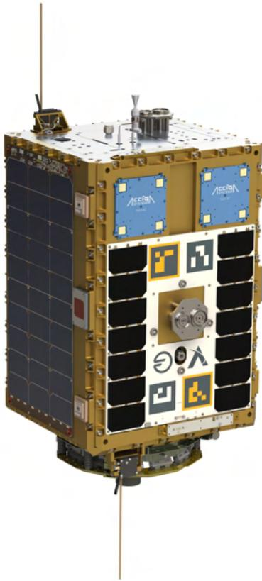
Fig. 1. Render of Tenzing's exterior including the spacecraft's two RAFTI interfaces and fiducials
