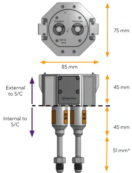
Fig. 14. RAFTI Block 2 Service Valve General Dimensions. Starred dimension may be adjusted for application requirements.
