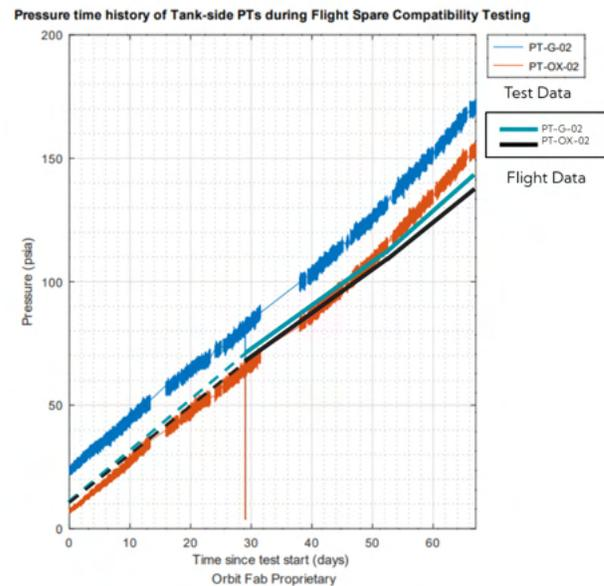
Fig. 13. Flight Spare and Tenzing Self Pressurization
