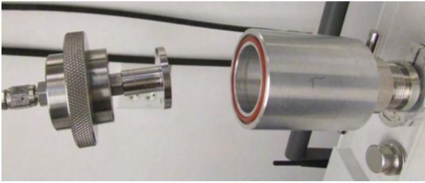
Fig. 8. Helium Leak test of RAFTI Block 0, unmated
