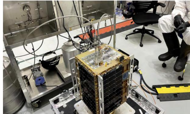
Fig. 12. Tenzing spacecraft with fill cart GSE lines installed
