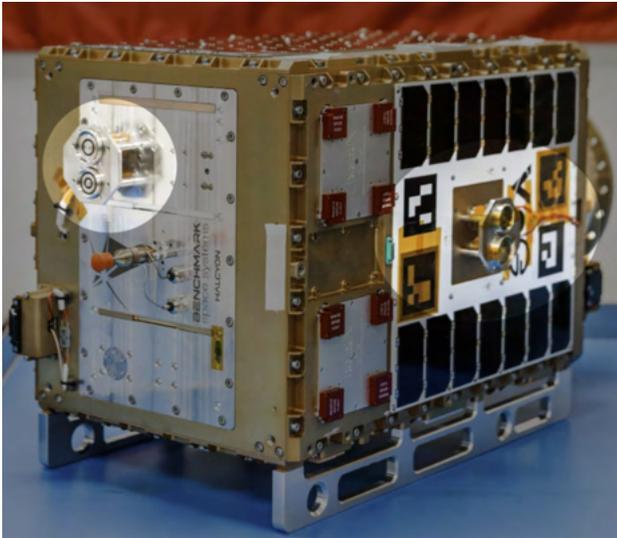
Fig. 11. RAFTI Block 1 Service Valves installed on Tenzing spacecraft
