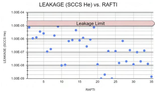
Fig. 7. Helium Leak test data for RAFTI Block 1
