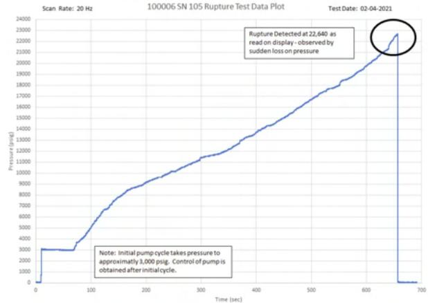
Fig. 10. Burst test data of RAFTI Block 0
